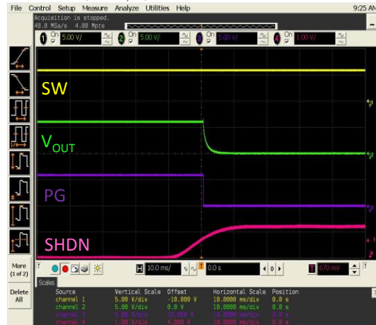
(6) Shutdown function Ta=25°C V_{IN}=6.0V , V_{SW}=V_{IN} , V_{SHDN}=0V \rightarrow 1.2V
