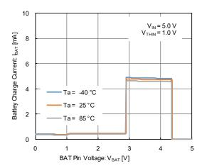
(4) Battey Charge Current vs. BAT Pin Voltage  $(R_{ISET} = 20 \text{ k}\Omega, \text{CV} = 4.35\text{V}, \text{Normal Operation})$
