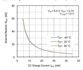
(2) CC Charge Current vs. Ambient Temperature (Normal Operation)
