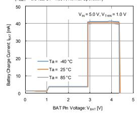
(6) Charge Completion Current vs. Ambient Temperature
