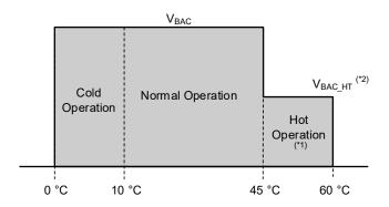
Constant-Voltage Charge vs. Thermistor Temperature
