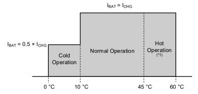
Constant-Current Charge vs. Thermistor Temperature
