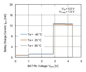
(5) Battey Charge Current vs. BAT Pin Voltage ( $R_{ISET}$  = 5.9 k $\Omega$ , CV=4.35V, Normal Operation)
