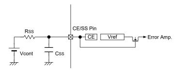
Ex.) Reference Circuit 1: N-ch Open Drain
