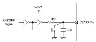
Ex.) Reference Circuit 2: CMOS Logic (Low Supply Current)
