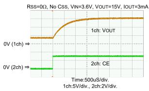
Ex.) When Css=0.1uF, Rss=220k $\Omega$ , Vcont=5V, t=-0.1×10<sup>-6</sup> × 220 × 10<sup>3</sup> × In((5-1.6)/5)=8.48ms
