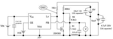
1. The measurement method of Lx On resistance RSWON Using the circuit ②, Lx On resistance can be measured by adjusting Vpull voltage to set Lx voltage VLx x 0.4V when the driver transistor is ON. The oscilloscope is used for measuring the Lx voltage when the driver transistor is ON.
