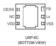
\*The dissipation pad for the USP-6C package should be solder-plated in recommended mount pattern and metal masking so as to enhance mounting strength and heat resistance. If the pad needs to be connected to other pins, it should be connected to the VSS pin.
