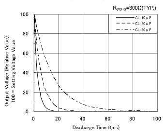
**Output Voltage Discharge Characteristics**
