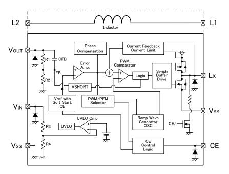
NOTE: The XCL201 offers a fixed PWM control, a signal from CE Control Logic to PWM/PFM Selector is fixed to "L" level inside. The XCL202 control scheme is PWM/PFM automatic switching, a signal from CE Control Logic to PWM/PFM Selector is fixed to "H" level inside. The diodes placed inside are ESD protection diodes and parasitic diodes.
