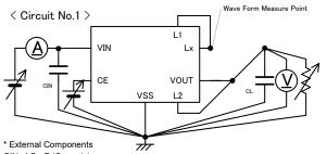
\* External Components CIN: 4.7  $\mu$  F (Ceramic) CL: 10  $\mu$  F (Ceramic)
