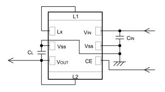
• External Components  $C_{IN}$  : 10V/4.7  $\mu$  F(Ceramic)  $C_L$  : 6.3V/10  $\mu$  F(Ceramic)
