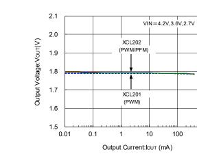
(2) Output Voltage vs. Output Current
