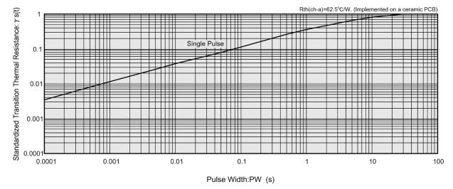
(11) Standardized transition Thermal Resistance vs. Pulse Width
