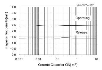
South Pole Magnetic Flux Density vs. Input Capacitance (CIN)
