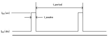
The Hall IC is operated intermittently to reduce supply current.
