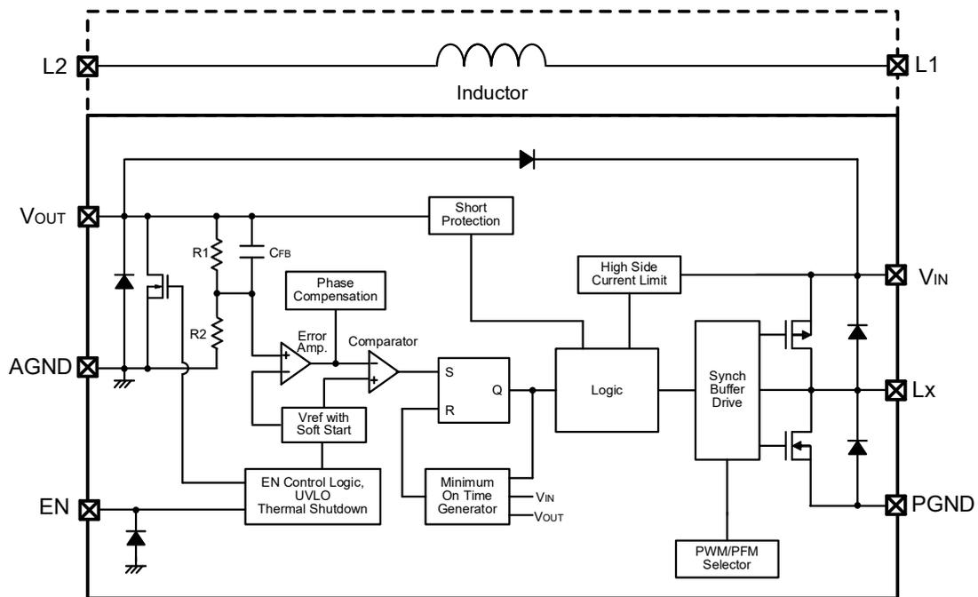
\*"PWM/PFM Selector" in the XCL241 series is fixed to PWM control.
