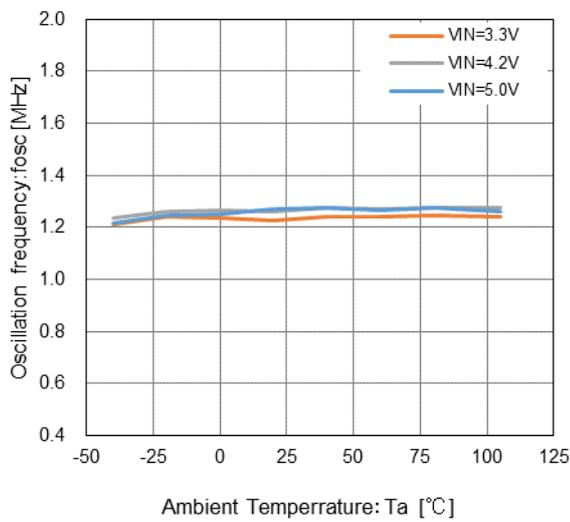
(13) Oscillation Frequency vs. Input Voltage
